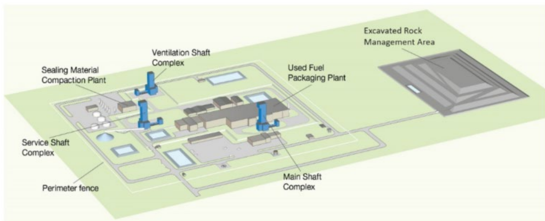
Figure 4-1: DGR Main Surface Facilities (NWMO, 2021b)
